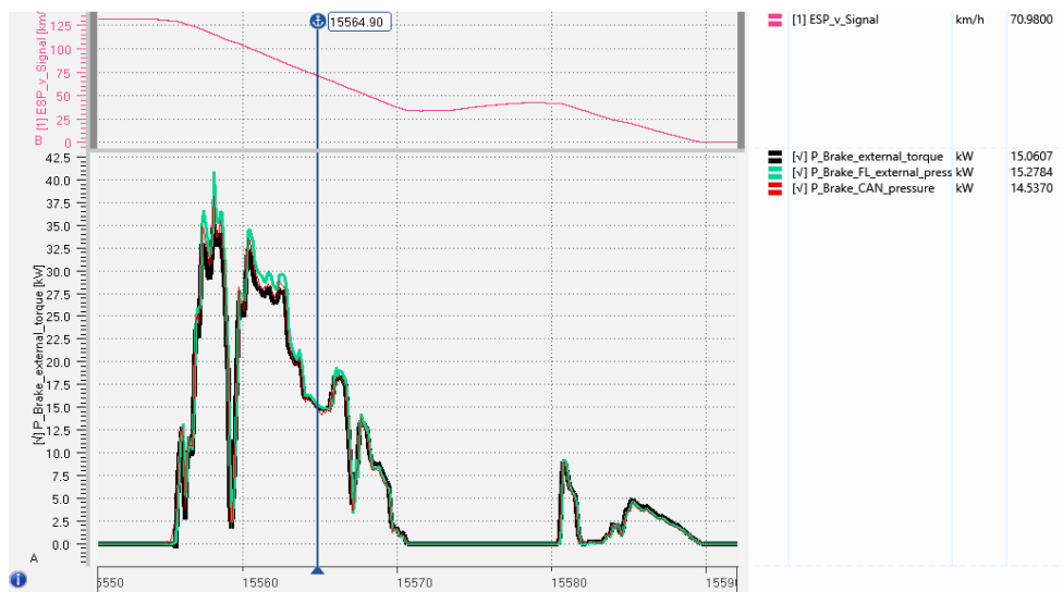
Figure B-2 Example comparison External Torque Sensor, External Pressure Sensor, and CAN based Pressure derived braking torque.
