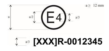
The above example of the approval mark shows that the concerned retreaded tyre has been approved in the Netherlands (E4) pursuant to UN Regulation No. [XXX], under approval number 0012345. The first two digits of the approval number (00) indicate that the approval was granted pursuant to the original form of that Regulation.
