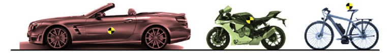
Fig. 2. CG positions of motorized vehicle, motor cycle, electric bicycle Image sources: Daimler, Yamaha, Merida
