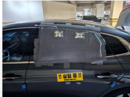
The outdoor air inlet and vent line
