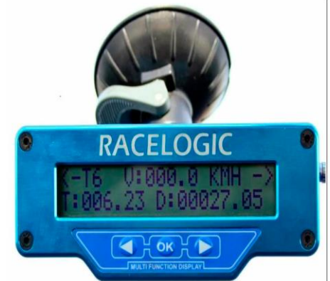
Vbox 3i Racelogic LTD for measuring distance, time, speed
