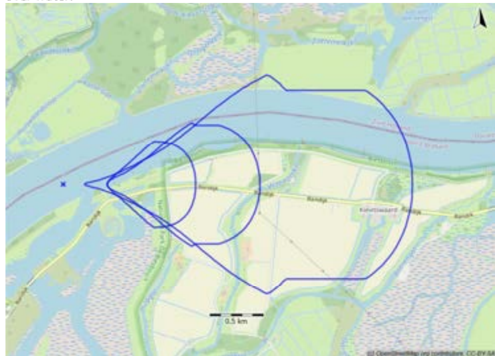
Figure 4.1 Propane – cloud fire contours for tank sizes 380, 1000 and 5000 m 3 .
