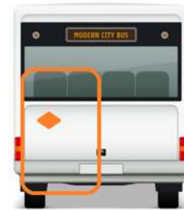
Figure 11.2 - Placement on a vehicle of categories M2 and M3
