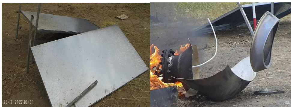
Figure 10: The witness plate and tank after test.
