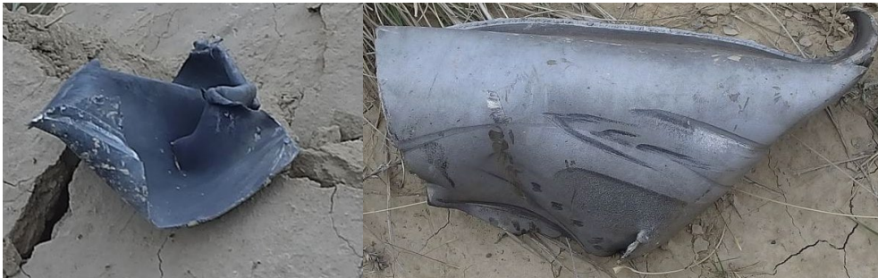
Figure 4: Fragments of the tank after the test.
