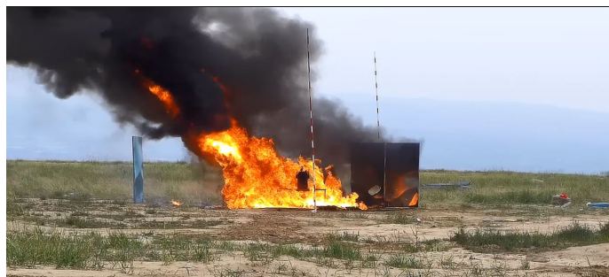
Figure 3: 20 L cylindrical stainless steel storage tank in the 6 (c) test.
