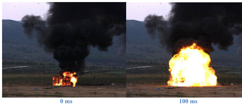
Figure 8: Hydrazine anhydrous packaged in 120 L cylindrical stainless steel storage tank.
