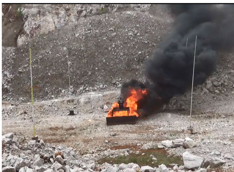
Figure 1: 20 L cylindrical stainless steel storage tank in the 6 (c) test.
