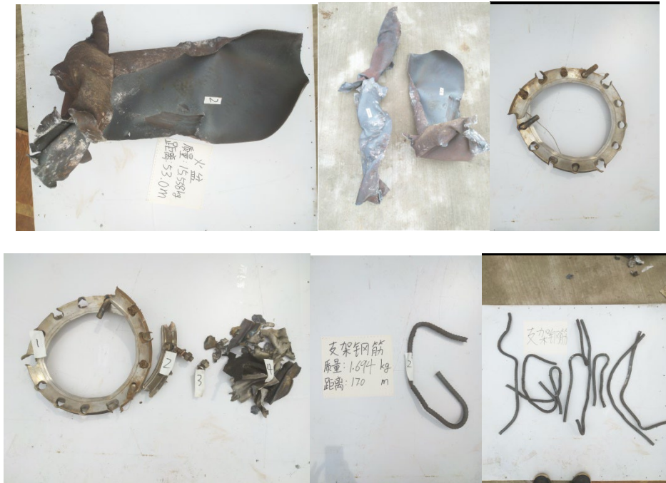
Figure 2: Fragments of the tank after the test.
