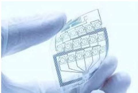
Figure 8 Flexible cellulose electronics
