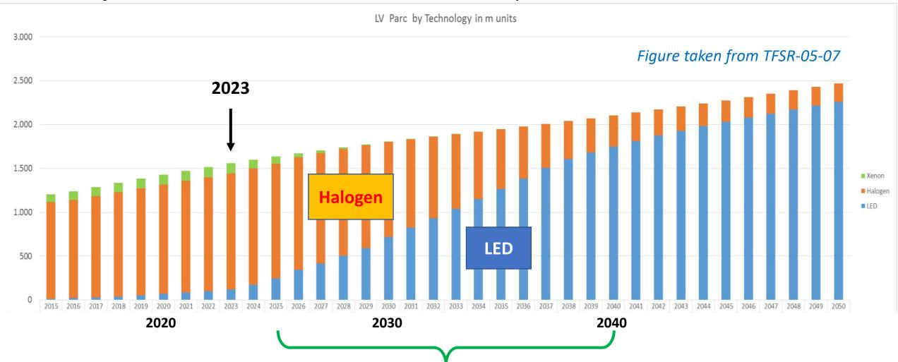
⇒ But, this transition can be accelerated by LED replacement solutions for vehicles in use
