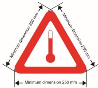
Figure 5.3.4: Mark for carriage at elevated temperature
