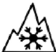
Minimum 15 mm base and 15 mm height when the marking is on the sidewall.
