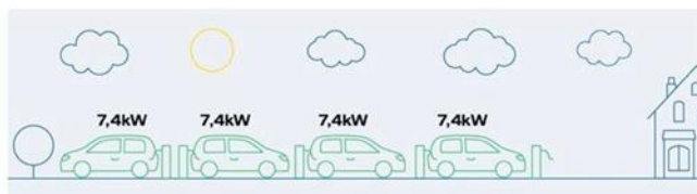
Figure III Dynamic Load Balancing with multiple charging stations
