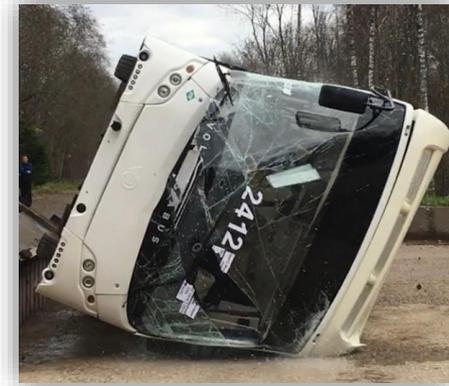
**A rollover test on a complete vehicle** was performed in accordance with the provisions of Annex 5 to UN Regulation No. 66-02.
