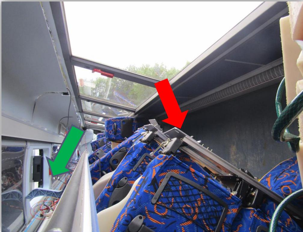
**Intrusion of individual structural elements (luggage racks) into the residual space of the vehicle**
