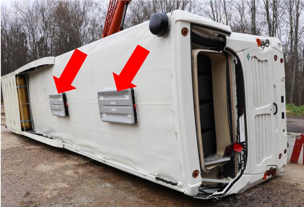
**The emergency hatches were failed to open in accordance with the instructions marked on them \***
