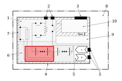
4. The safety system that is part of high voltage batteries is often designed to protect against an external short-circuit. As a result, test is passed without current flow, because the protective components, (red shaded box in illustration 6 above) are preventing it, via a fast reaction-rate open-circuit disconnect. This is the best technical way to prevent the risks related to the application of an external short circuit.
