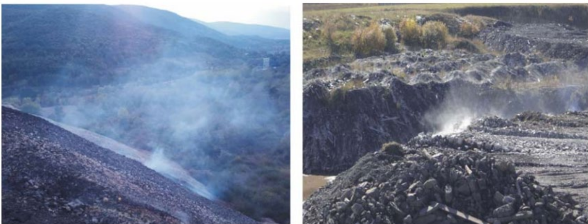
Figure 1.7 - The appearance of spontaneous combustion of coal in RMU "Soko" waste piles (left-hand side photo) and RMU "Štavalj" waste piles (right-hand side photo)
