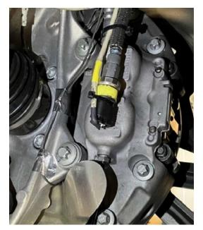
Method D: With internal Torq equiv. sensors and the brake torque is CAN output
