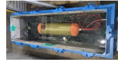
Bus Hydrogen Storage container Residual burst strength test
