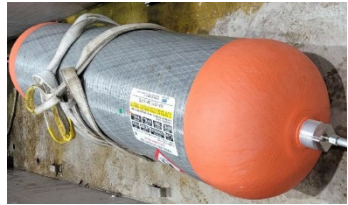
Bus Hydrogen Storage container Before HTSPT
