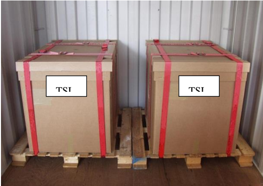
Figure 7.11 Cargo firmly secured to pallets by textile lashings, transport stability level marked
