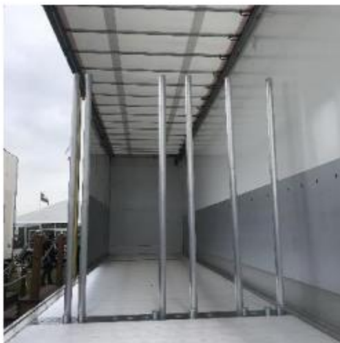
Figure 7.14 Floor mounted stanchions
