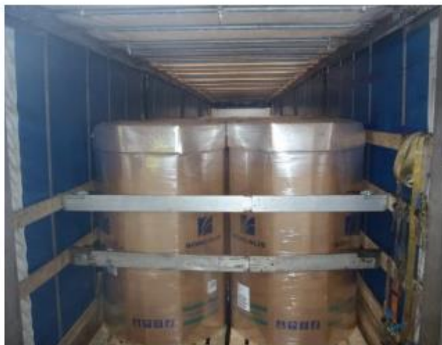
Figure 7.15 Blocking cross beams
