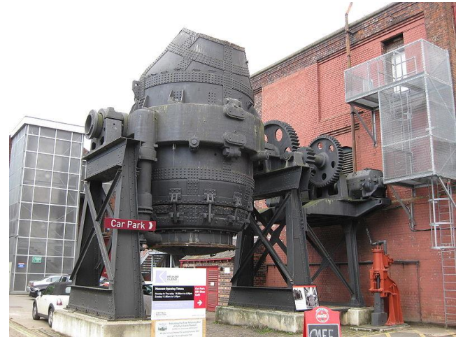
Bessemer converter, the most important technique for making steel from the 1850s to the 1950s, Sheffield (credits: Wikipedia, Chemical Engineer)
