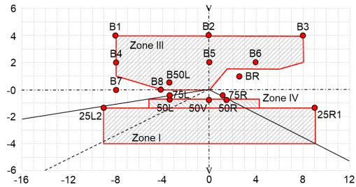
The test point locations for left-hand traffic are mirrored about the VV line"
