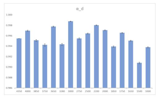
Evaluation of the impact on the pressure sensor accuracy at the intake (fictive engine) with  $\pm 800$  mbar: Pa
