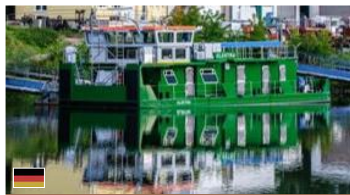
Push boat with Hydrogen Fuel Cell and batteries (Elektra)
