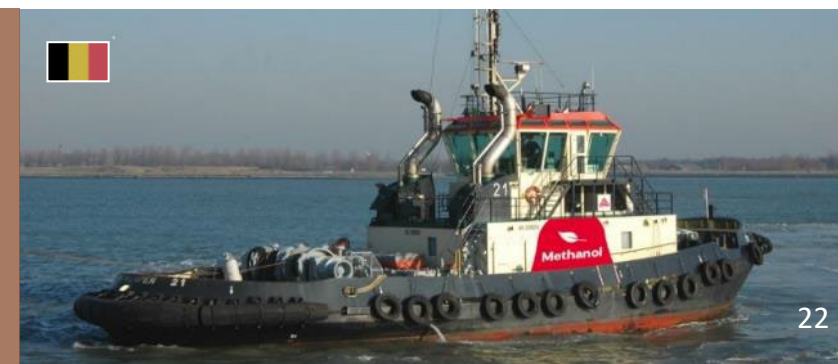
Port of Antwerp – European Fastwater (tugboat conversion to diesel-methanol propulsion)
