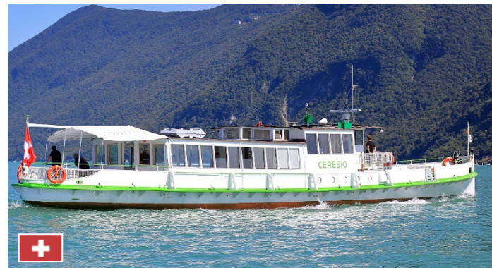
Retrofit of 1931 passenger vessel with batteries (MNE Ceresio)
