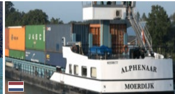
Vessel with exchangeable battery containers for propulsion
