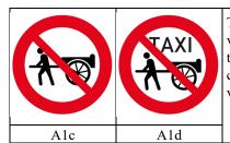
The sign under [A1c] would forbid entrance for all 'hand drawn or pulled vehicles', while [A1d] does not allow for 'hand drawn or pulled vehicles transporting passengers'. How could access be prohibited for such vehicles carrying goods? The use of Symbol [A1] would be insufficient, due to lacking visual differentiation to [A1a] (see 3).
