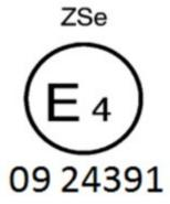
The belt bearing the above approval mark is part of a restraint system ("Z"), it is a special type belt ("S") fitted with an energy absorber ("e"). It has been approved in the Netherlands (E 4) under the number 0824391, this Regulation already incorporating the 06, 07, **08 or 09** series of amendments at the time of approval.
