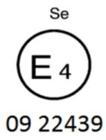
The belt bearing the above approval mark is a special type belt ("S"), fitted with an energy absorber ("e") and approved in the Netherlands (E 4) under the number 0822439, this Regulation already incorporating the 06, 07, **08 or 09** series of amendments at the time of approval.
