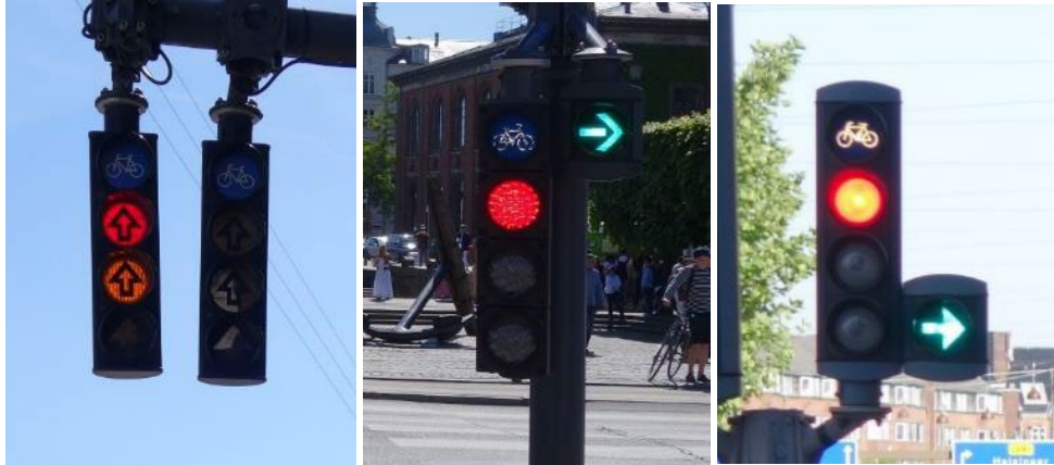
Figure 4. Examples of directional traffic lights with a panel (?) indicating that the signals are dedicated for cyclists (Denmark).
