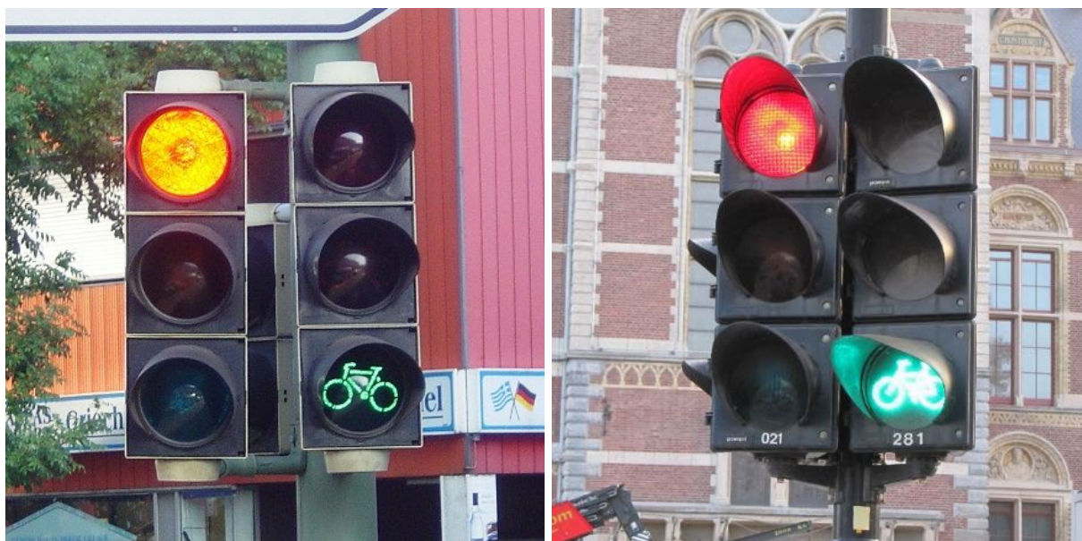
Figure 3. Traffic light signals with a red, amber and green symbol of cycle on black background are clear and exclude any possibility of being mistaken by drivers for light signals for other traffic. Examples from Germany (left) and Netherlands (right). Source respectively: Marcin Jackowski and Aleksander Buczyński
