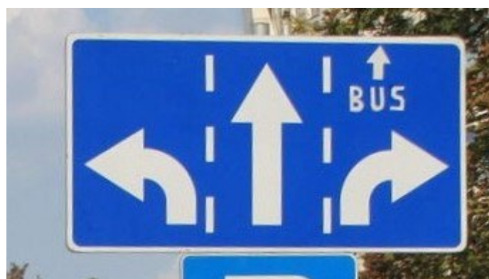
Figure 9. Example of different lane selection for different groups of users: busses are allowed to go straight from the right-turning lane, because of a bus-and-cycle lane starting after the intersection. Source: Aleksander Buczyński
