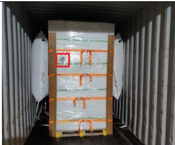
Figure 1. Package containing lithium ion batteries affixed the label model No. 9A (100 mm × 100 mm) in a container
