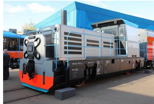
Hybrid battery-trolley DC electric locomotive with induction motor drive and on-board energy storage
