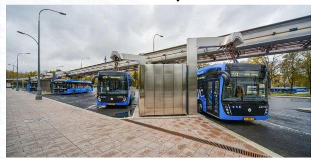
Separation of tracks with markings and stone barriers Construction of tram platforms at the same level with tram floor 40-50 km of range after 8-10 minutes charging at terminus 200 charging stations now working + 200 more by 2024 The largest electric bus depot in Europe for 300 vehicles
