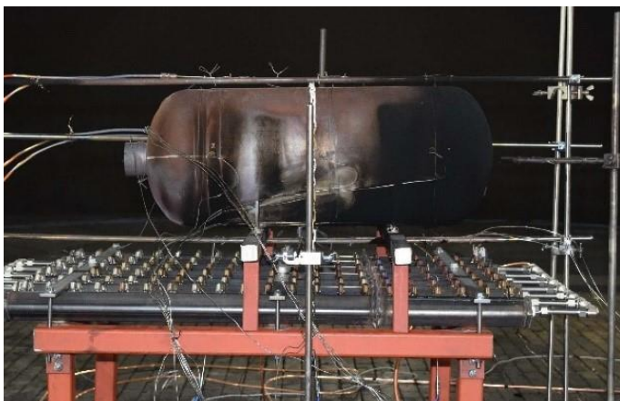
Figure 18 Pre-Test Cylinder Mounted Above the Burner for Thermal Mapping
