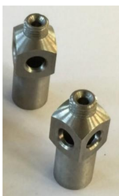
Figure 16 Burner Fuel Nozzles
