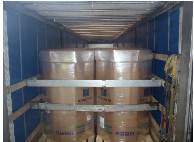
Figure 7.15 Blocking cross beams
