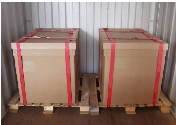
Figure 7.8 11 Cargo firmly secured to pallets by textile lashings
