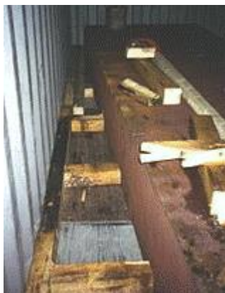
Figure 7.4561 Transverse blocking of steel slab
