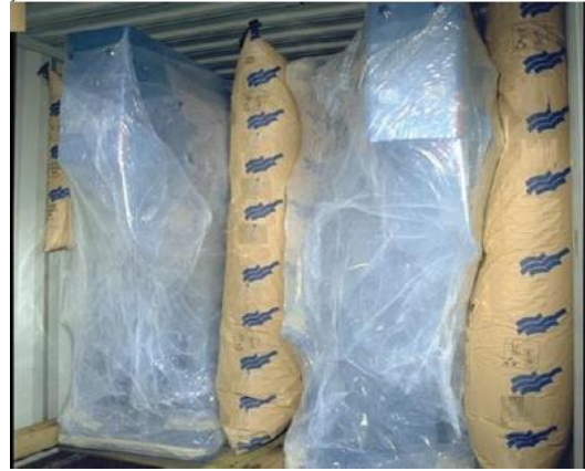
Figure 7.913 Irregular shaped packages blocked with dunnage bags
