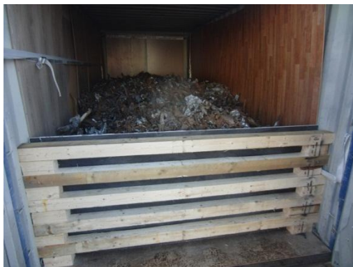
Figure 7.5574 Lined container CTU with liners and door barrier loaded packed with scrap
