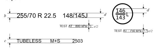
(<sup>2</sup>) "TEST AT :" may be replaced by "TEST INFL :" or the symbol "@" or be omitted.
