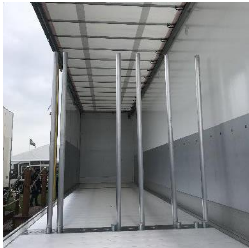
Figure 7.418 Floor mounted stanchions
