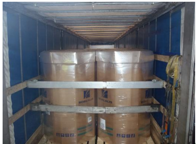
Figure 7.5 Blocking cross beams
