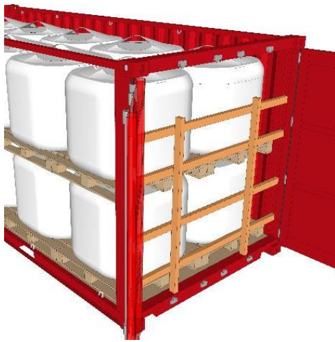
Figure 7.40 Shoring bars inserted in the shoring slots and supported by uprights placed against the doors
