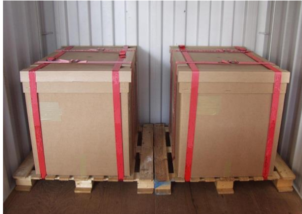
Figure 7.8-165 Cargo firmly secured to pallets by textile lashings
