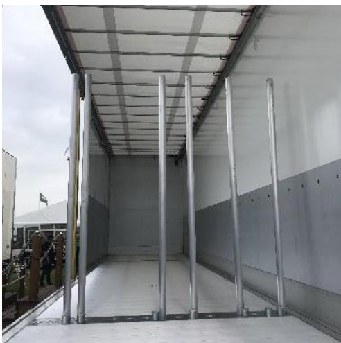
Figure 7.4 Floor mounted stanchions
