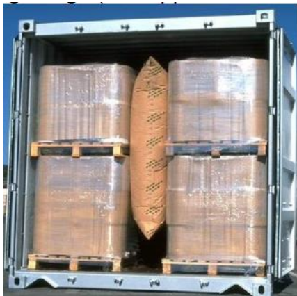
Figure 7.176 Gap filled with central dunnage bag
