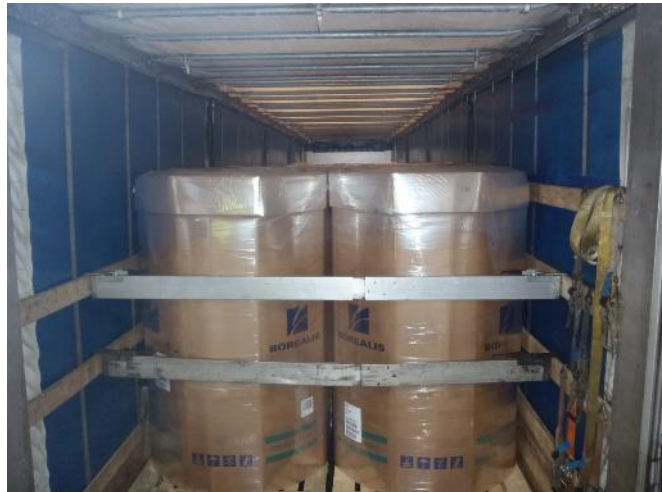
Figure 7.519 Blocking cross beams
