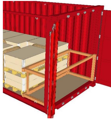
Figure 7.41 Cross beams inserted in the corrugations supported by shoring beams against the doors at the hinges
