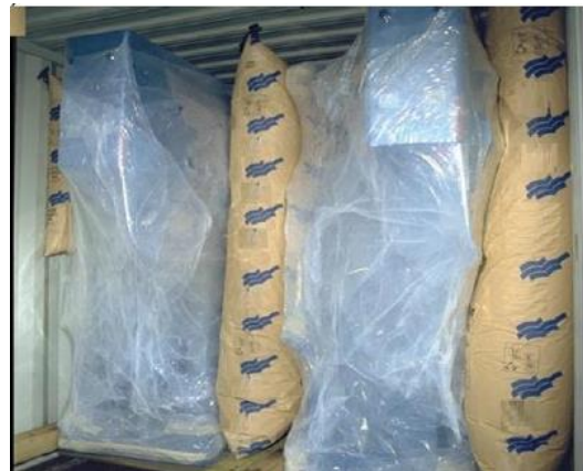
Figure 7.187 Irregular shaped packages blocked with dunnage bags
