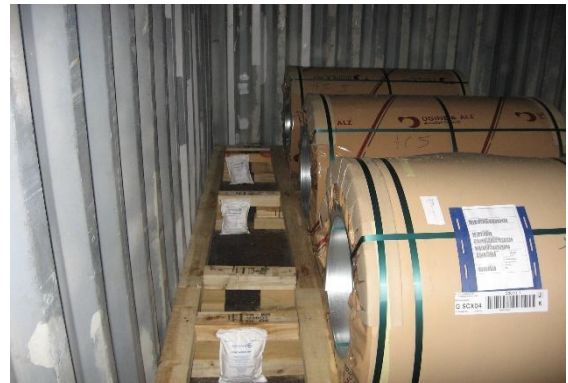
Figure 7.36 Boundary blocking arrangement
