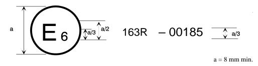
The above approval mark affixed to a vehicle shows that the type concerned was approved in Belgium (E 6) pursuant to UN Regulation No. 163. The first two digits (00) of the approval number indicate that the approval was granted in accordance with the requirements of UN Regulation No. 163 in its original form.
