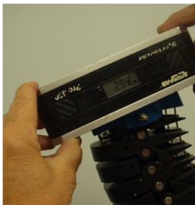
Figure 53 Occipital Condyle Plate angle setting
