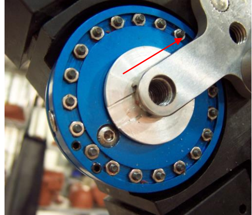
Figure 11 Slide damper into place
