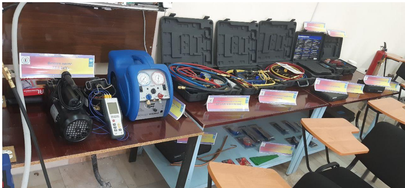
Figure 12. Special tools for servicing refrigeration equipment
