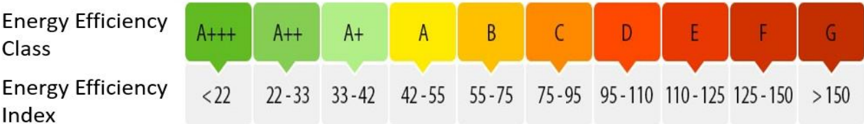
Figure 4. Classification of refrigerators in accordance with the energy efficiency index
