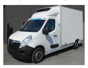
Case No. 4: Standard production vans with integrated insulation and the unit installed under the chassis or in the engine compartment:
