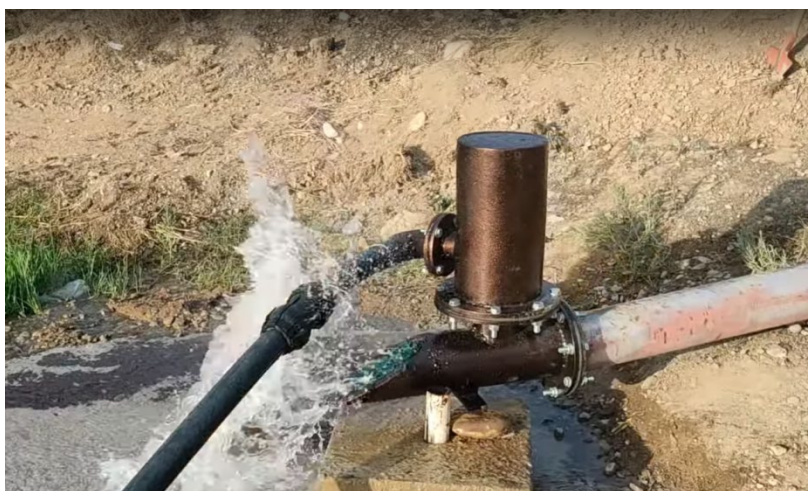
Figure 12 Improved hydraulic ram pump of Rogozin
