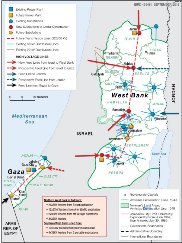
Map A.1: Electricity Supply System in the West Bank and Gaza
