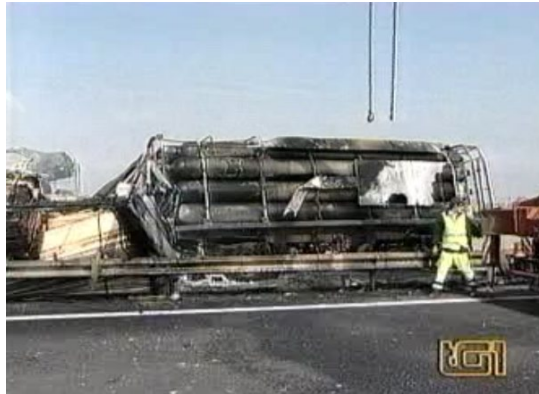
Fig. 1: 2003, Italy, full fire engulfment, no catastrophic failure.
