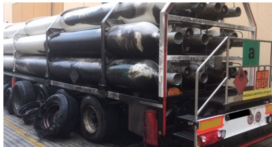
Fig. 3: 2019, Italy, tyre fire, no leakage, no rupture
