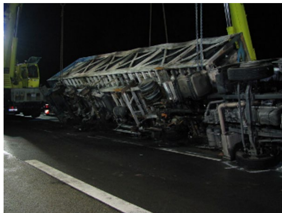
Fig. 2: 2009, Germany, full fire engulfment, leakage of some but not all elements, no rupture
