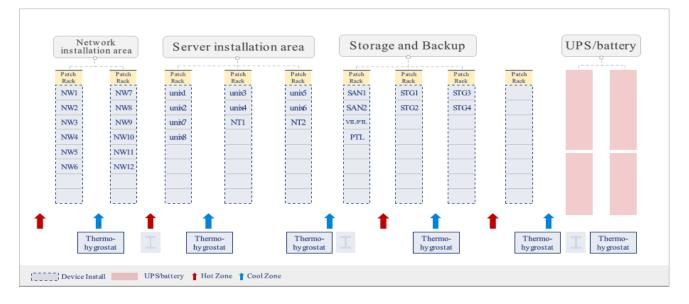
Table 15 provides an example of calculating the required rack unit (RU), assuming that one rack in the IDC can accommodate standard 42 RUs. The example shows that the network requires a total of 162 RUs. Adding 50 per cent of free
