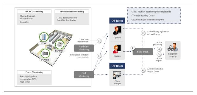
The facility management system can also process the fault handling and notification to corresponding clients. Based on operators' analysis of the fault, it will be processed accordingly, which may involve maintenance work carried out by the operator, or the dispatch of engineers and equipment suppliers (Figure 28).
