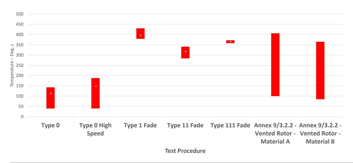
Annex 9 / 3.2.2. tests with vented rotors broadly cover the temperature spectrum seen on R90 Approval tests
