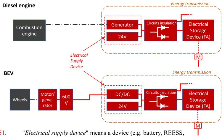
2.51. "Electrical supply device" means a device (e.g. battery, REESS, DC/DC converter, generator, fuel-cell or a combination of those components) that supplies electrical energy to the braking system's electrical energy storage device(s).
