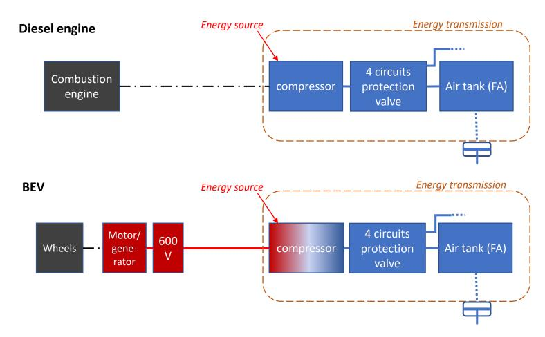
2.49. "Energy source" means a device that both generates and provides energy required for the braking system.
