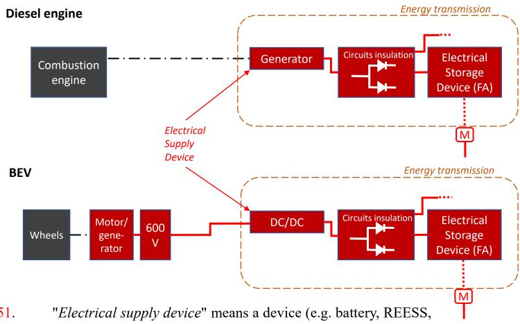
2.51. "Electrical supply device" means a device (e.g. battery, REESS, DC/DC converter, generator, fuel-cell or a combination of those components) that supplies electrical energy to the braking system's electrical energy storage device(s).
