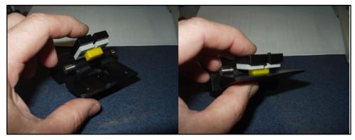
Remove the two M2.5 SHCS that retain the T1 pin at the C7-T1 joint (Figure 82). Slide the T1 pin out of the vertebrae joint (Figure 83) and set it aside along with the two M2.5-0.45 x 8 SHCS for re-installation later."
