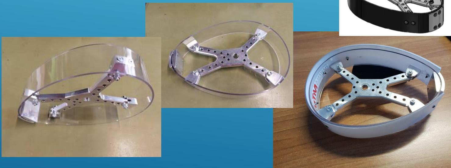
Other polycarbonate layers of different thicknesses can be superimposed on the base frame to achieve the desired stiffness. The outer layers can be easily replaced in case of damage in the surface friction test.
