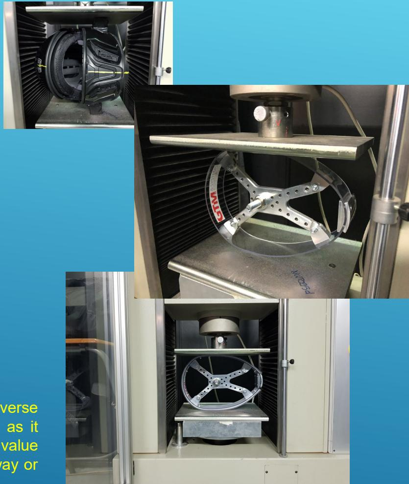
The simulacrum has about the same longitudinal and transverse stiffness of a helmet, the stiffness represents a compromise as it would be anyway because it is impossible to have an exact value that can represent full/modular and jet helmets in the same way or in composite or plastic material.
