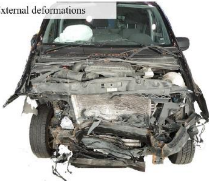
Figure 5: External deformations on the van and the interior of the passenger compartment. Illustration/photo: NSIA
