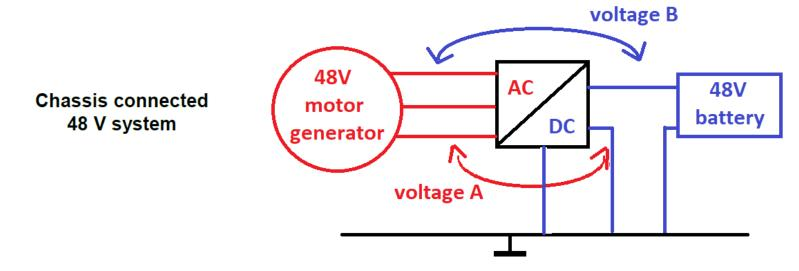
\* Voltage B between a DC life part (e.g. B+ bolt of an 48V Motor Generator (MG)) and an AC live part (e.g. phase of an 48V MG) has been not considered so far in the referenced document (see above). Voltages A and B can be evaluated as composite/mixed voltage and would in that case be > 30V AC (rms), which would be in conflict with the "specific voltage condition" in ECE-TRANS-WP.29-GRSP-2020-06e, paragraph 2.4.
