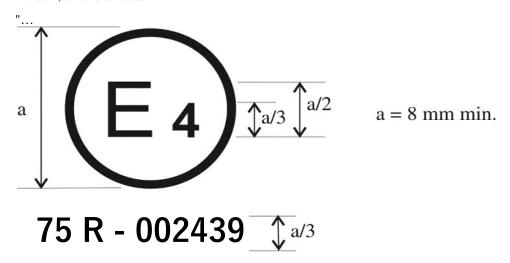
The above approval mark affixed to a tyre shows that the type of tyre concerned has been approved in the Netherlands (E 4) pursuant to UN Regulation No. 75 under approval number 002439. The first two digits of the approval number indicate that the approval was granted in accordance with the requirements of UN Regulation No. 75 in its original form.
