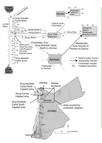
**Direct reuse**: Wastewater treatment plants effluent is used in the vicinity of the treatment plants for irrigation of fodder crops and trees.
