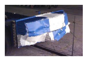
Figure 12 Cellbond MDB Face, after Vehcle A Test
