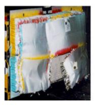
**Figure 13** EuroNCAP MDB Face after Test with Vehicle Model A.
